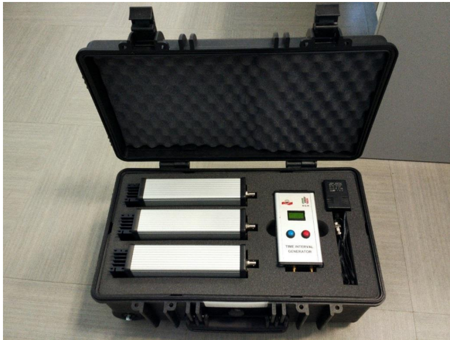
Fig 3. Case for the travelling standards containing 3 InLambda standards, TIGen standard – base unit and power supply adapter for TIGen standard
